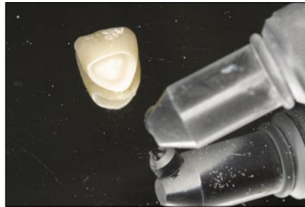
Figure 9. Microsandblasting with 50µm Al 2 O 3 particles.
